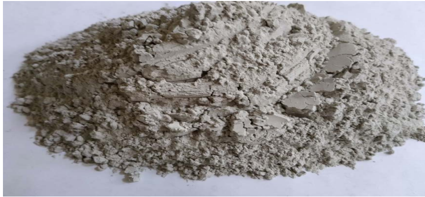
Figure 9: Granite Powder as an Alternative Cementing Material
