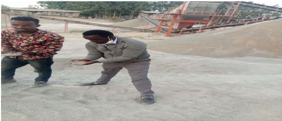
Figure 10: Crusher dusts from Hawassa Monopol as fine aggregate
