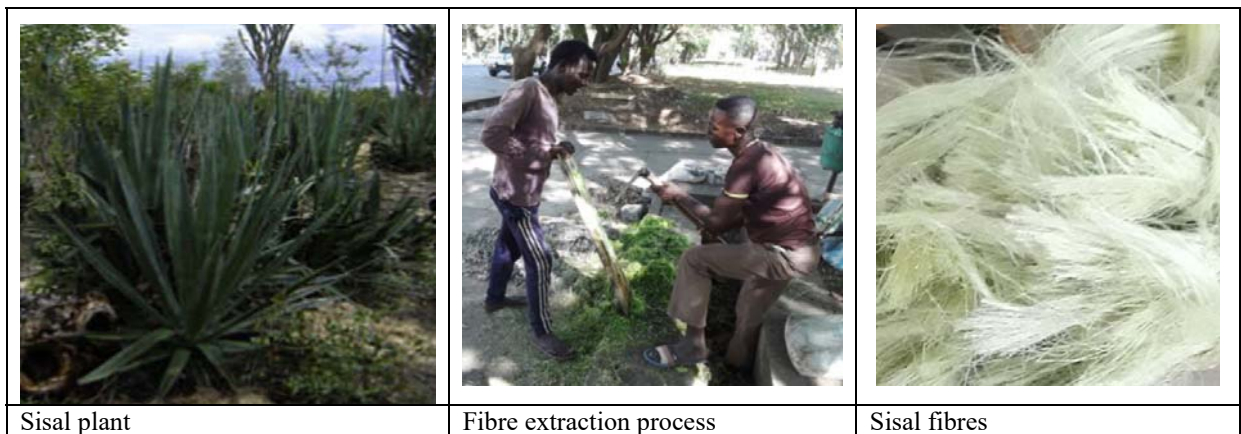
Figure 8: Sisal fibre a natural fibre for arresting tensile cracks in concrete
