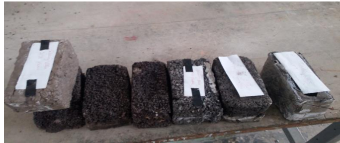
Figure 6: samples of bricks made from molten plastic and the three materials.
