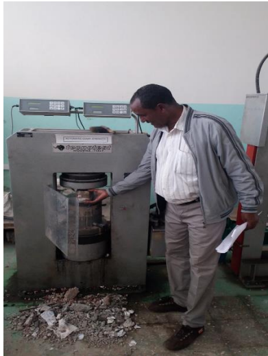
Figure 8: Compressive strength test
