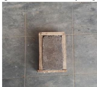
Figure 5: Wooden mold used to cast the bricks
