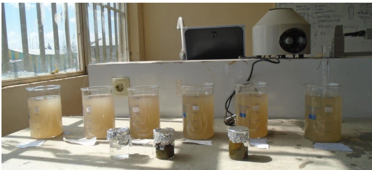
Figure 2: Experiment on coagulation using different doses and alum as a control.
