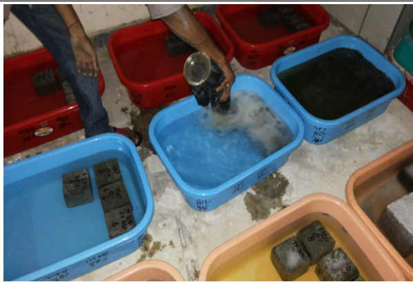
Figure 6: Acids Attack Testing
