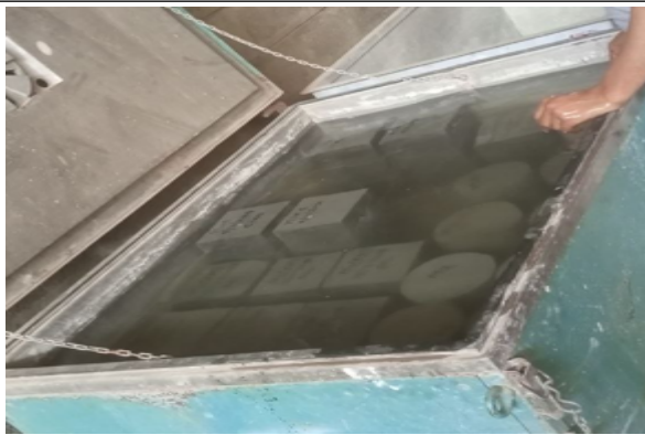
Figure 4: Curing of Concrete Specimens
